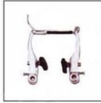
MOD: BK-030 ALUMINUM V-BRAKE ARMS LENGTH: AVAILABLE IN 105mm & 100mm STANDARD FINISH: SILVER OR EDBACK COLOR OPTIONS: ANODIZED OR PAINTED TENSIONING: COIL SPRING RUBBER PAD: 55-72mm AVAILABLE
