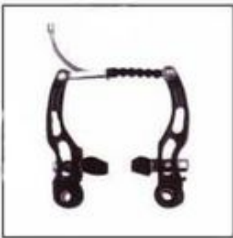
MOD: BK-050 STEEL V-BRAKE ARMS LENGTH: 98mm STANDARD COLOR: CP OR EDBLACK COLOR OPTIONS: ACCORDING TO ORDER TENSIONING: COIL SPRING RUBBER PAD: 55-72mm AVAILABLE
