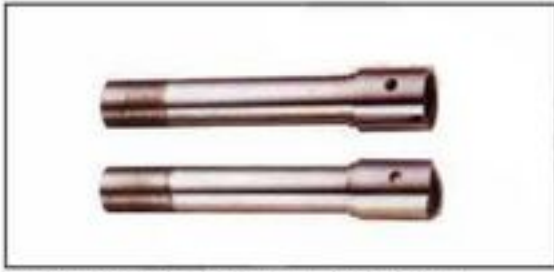
MOD: CP-01 FORK HEAD STEM MATERIAL:STKM11A T:BC1"X24T L:160mm-300mm
