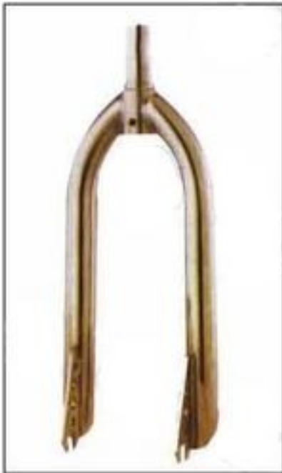
MOD: NK-01 TYPE:FOR BMX SIZE:12", 16", 20" ITEM:1"or 1-1/8" BLADES:1", 1-1/8 or 1-1/4" ENDS:T4mm PRESSED ENDS FINISH:CP or PAINTED
