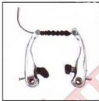
MOD: BK-060 STEEL V-BRAKE ARMS LENGTH: 105mm STANDARD COLOR: CP OR EDBLACK COLOR OPTIONS: ACCORDING TO ORDER TENSIONING: COIL SPRING RUBBER PAD: 55-72mm AVAILABLE
