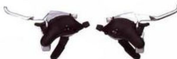
MOD:DLF-08 Twist index shifter with braker lever. Feature:3 finger alaminum alloy braker lever. Clamp diam:Φ22.2mm Left:Friction, 3 spd index Right: friction,5,6,7,8 spd index
