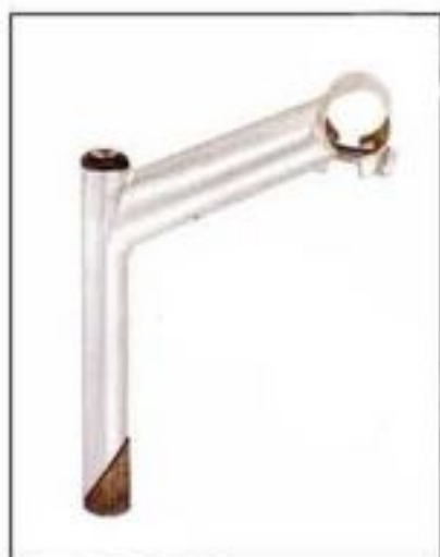
MOD:HS-01 MATERIAL:STEEL EXT:90mm-130mm RISE:0DEG-55DEG FINISH:BED/AP
