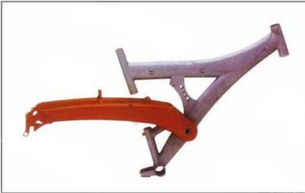
MOD:SF-01 SUSPENSION FRAME TYPE:26"SINGLE STAY TYPE MATERIAL:STEEL SHOCK:ALLOY or STEEL FINISH:PAINTED H/T:34X30X120mm T/T:50.8X1.4mm D/T:60X1.4mm S/T:31.8x1.4mmX18" B/B:40X68mm
