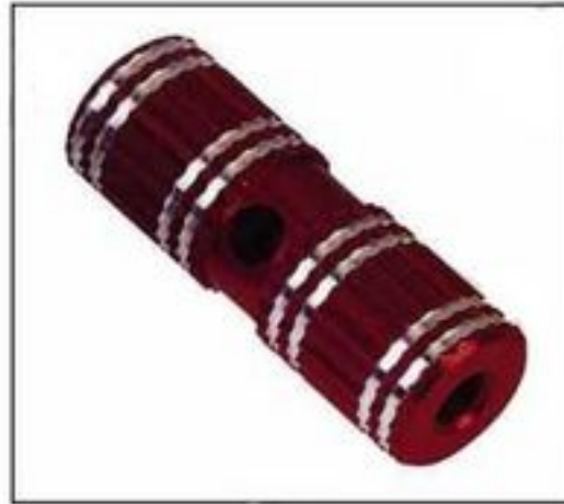
Mod: TG-Y06A-02 Step Peg Diameter: \Phi 20 - \Phi 28 Length: 70-110mm Thread: 3/8"X24T 26T 10X1 Color: To order
