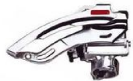
MOD:DRN-18 Index front derailleur down pull Suitable for triple or quadruple chainwheel Steel clamp diam: 1-1/8", 1-1/4" Capacity 22T, top gear 48T
