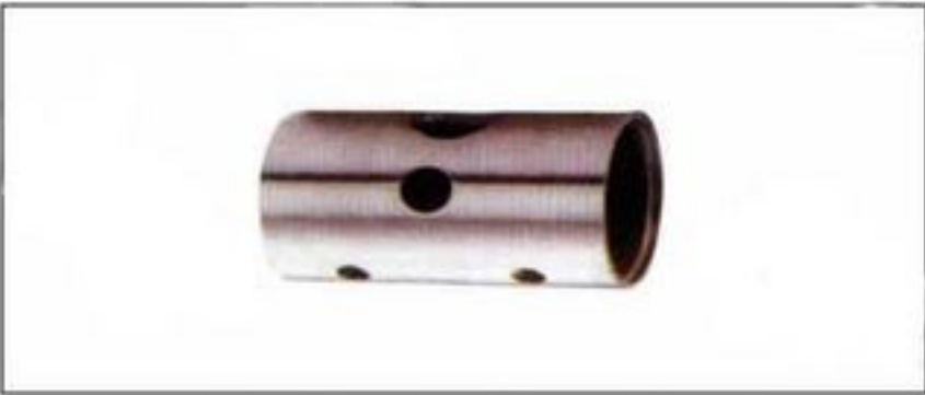
MOD: LS-03 BOTTOM BRACKET SHELL MATERIAL:STKM11A BC:1.37X24T OD:40mm ID:34mm LENGTH:65-73mm
