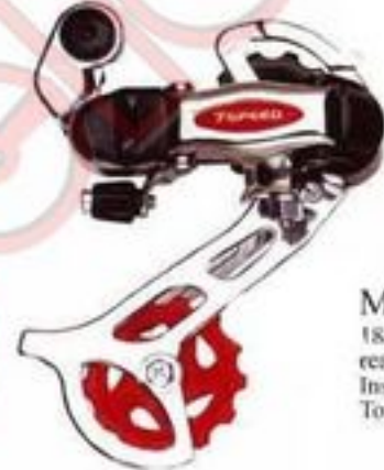
MOD:DRN-14 15/18 Speed index rear derailleur, long cage Installation: directly Total capacity: 36T
