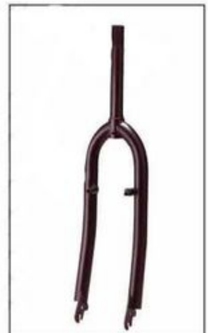
MOD: NK-10 FOR MTB UNICROWN TYPE STEM:ID 21.1mm, 22.2mm OR 25.4mm BLADE:1-1/4 OR 1-1/8" (ROUND) END:PRESSED ENDS
