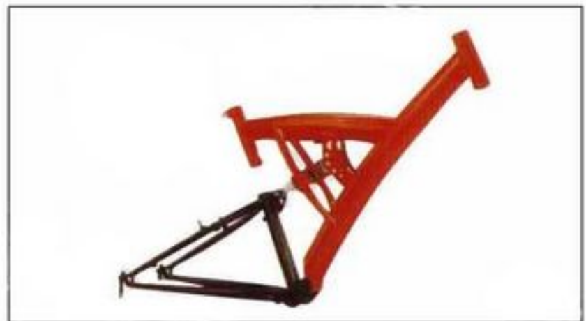
MOD: SF-05 SUSPENSION FRAME TYPE: 26"Y-TYPE MATERIAL: STEEL SHOCK: ALLOY or STEEL FINISH: PAINTED T/T&D/T: 60X1.4mm
